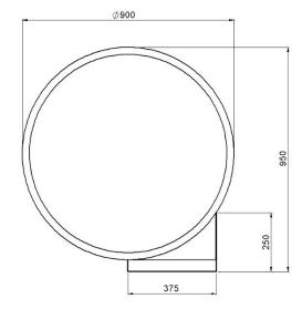
Dimensions: Φ900 x 950 mm Total power:90w Luminaire luminous flux: 9000lm Luminaire efficacy: 100 lm/w Weight: 4.5 kg
